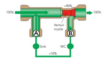
**Figure 18(b)** Section through a KHS-Multi-Circ Standard Distribution Unit (incorporating a venturi nozzle) creating a flow in an otherwise stagnant supply loop.
