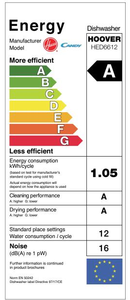
**Figure 14** Example of an energy label from dishwasher packaging showing an ambiguous capacity and water consumption declaration.
