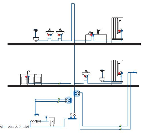
**Figure 20** Example of a water supply layout in dwelling with high use kitchen sink, showers and WC, but low use external taps. All terminal branches are kept as short as possible. The vertical loop on the upper floor is for a future extension of the water supply system.
