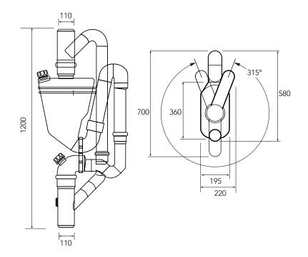
Figure 22 A drain booster vertical syphon for installation near the base of a stack (all measurements in millimetres).
