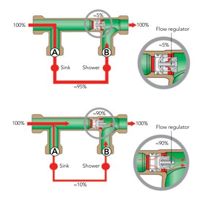
**Figure 19** Sections through a KHS-Multi-Circ Dynamic Distribution Unit, incorporating a venturi flow regulator, showing the impact of different flow volumes through the main branch on the circulation within the loop.
