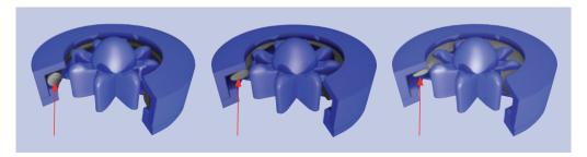
**Figure 9** The components of a pressure-compensating flow limiter, showing the O-ring moving and deforming under different pressures.
