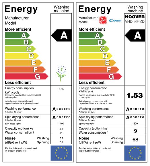
**Figure 12** Washing machine energy label, including ecolabel flower symbol, dry load capacity and water consumption in litres for a 60°C cotton wash.
