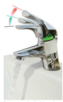
**Figure 2** Section through a click tap with a water brake.
